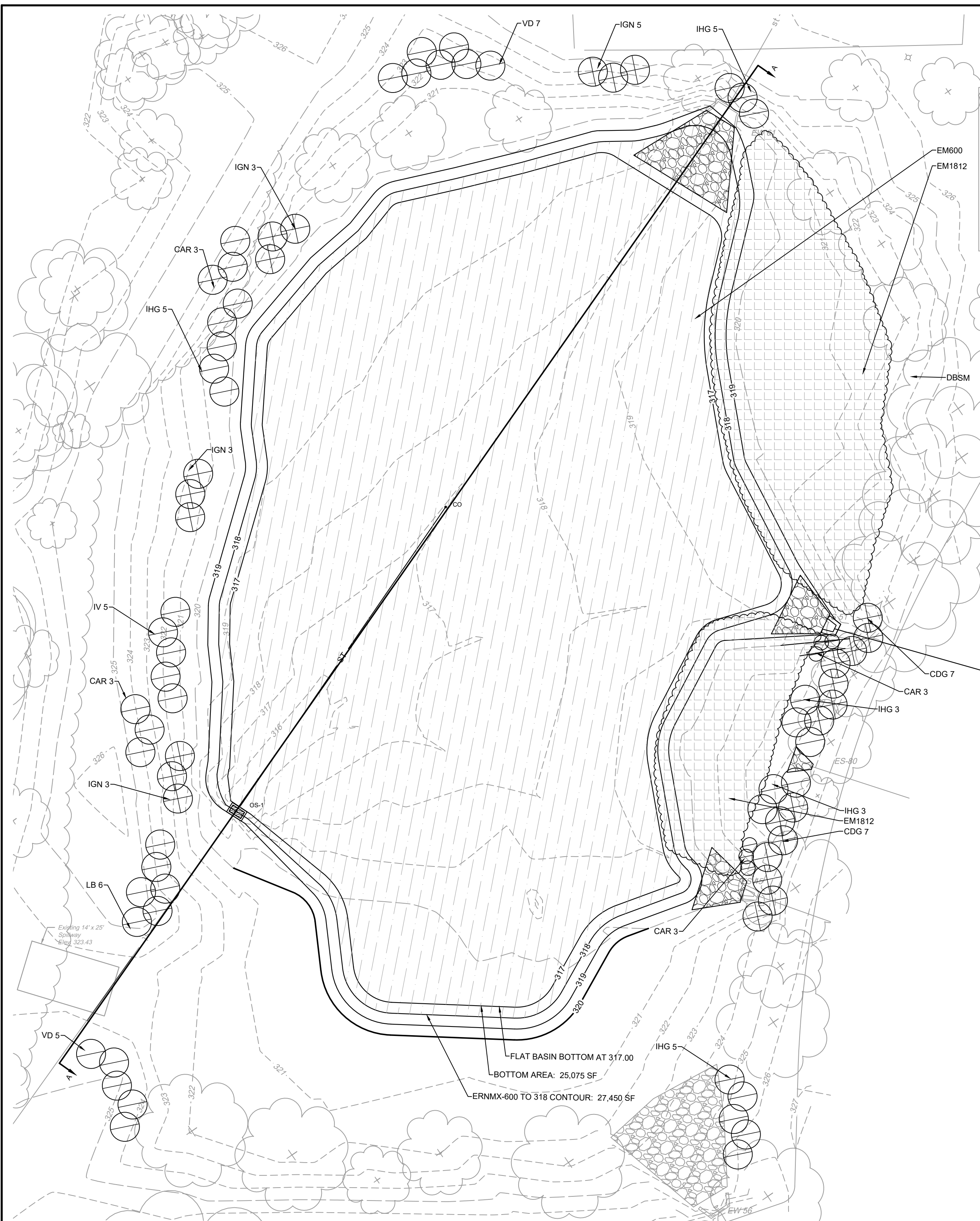
BMP-1 INFILTRATION BASIN PLAN VIEW SCALE: 1" = 20'
